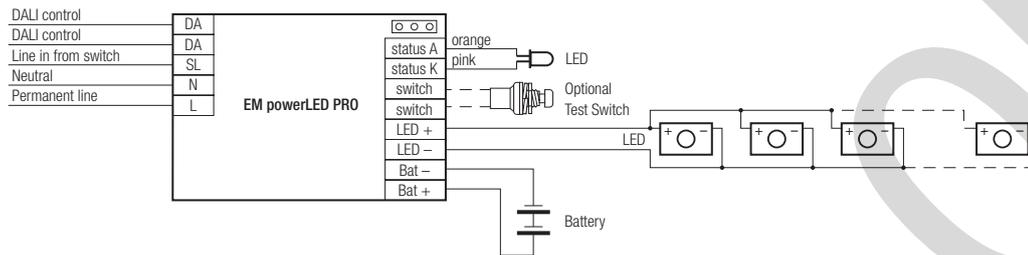
Take care that the LED is connected with the right polarity. LED that are connected to the EM powerLED devices should have a reverse polarity protection device such as a schottky diodes fitted, otherwise irreversible damage could occur if the LED is connected in reverse polarity. Any protection device must be capable of handling in excess of 700 mA.
